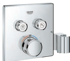
29 125 000 + 35 600 000 Grohtherm SmartControl thermostat for concealed installation with 2 valves and integrated shower union + separate concealed body
